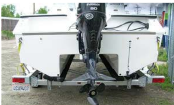
Port Erie tunnel and 26° dead rise angle of bottom.
