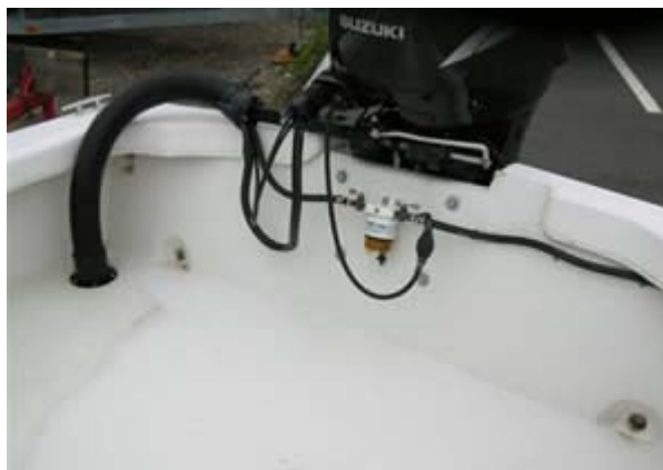
Aft section of one of the best selling cats. It has no aft bulkhead or splash well.
