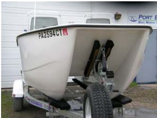
Port Erie Catamaran bottom. Note fullness on bow section and vertical tunnel.
