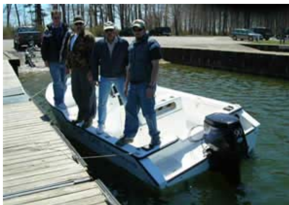
Splash well and aft bulkhead. Bulkhead is notched to let the motor tip up fully.
